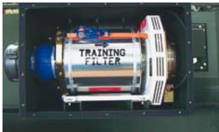
■ Bioquell MDH AFV training filter. Single-pass systems need regular filter changes
